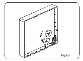
4.Put the battery into the installationsite and make sure the positive side of the battery is in accordance with the positive side of installationsite.(See Fig.3-3)
