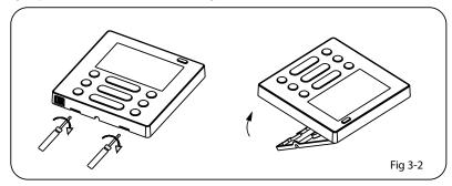
3. Take off the cover of wire controller at the bottom with the screwdriver. (See Fig.3-2)
